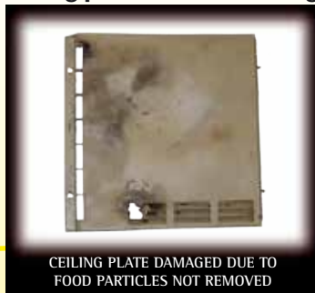
Ceiling plate burnt or missing
